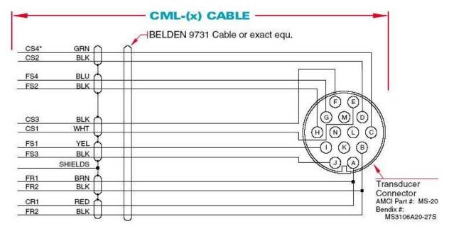
\*Industry standard resolver designations. The "F" or "C" prefix refers to the Fine or Coarse resolver in the transducer. The Fine resolver yields the position with in the turn, while the difference in position between the Fine and Coarse resolvers yields the number of turns completed.
