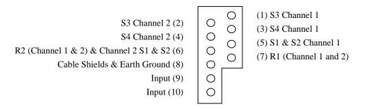
Make the following connections to simulate the resolvers of either channel at its 90 degree point. PLEASE NOTE, ONLY ONE CHANNEL AT A TIME CAN BE SIMULATED.
