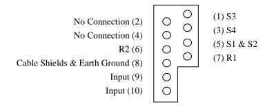
Make the following connections to simulate a resolver at its 90 degree point.
